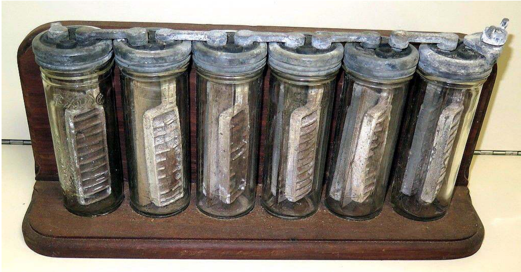
An example of a 1920s lead-acid radio storage battery assembly
