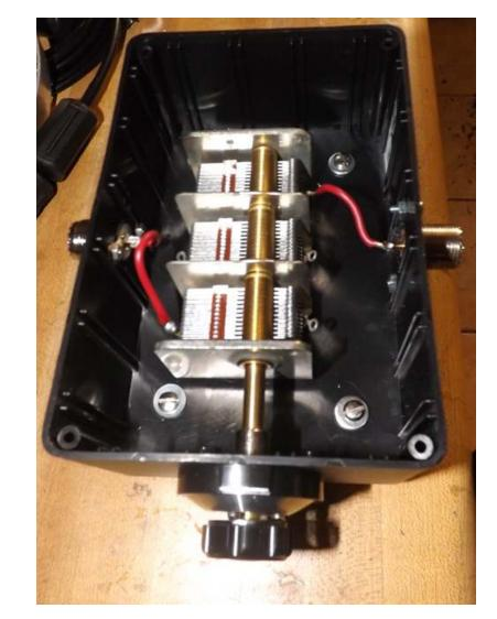
Contrary to conventional wisdom, the center and shell of the SO-239 connectors are shorted with grounding lugs. This is because both the shield and inner conductor of the LMR-400 cable are tied together to form the large loop.
