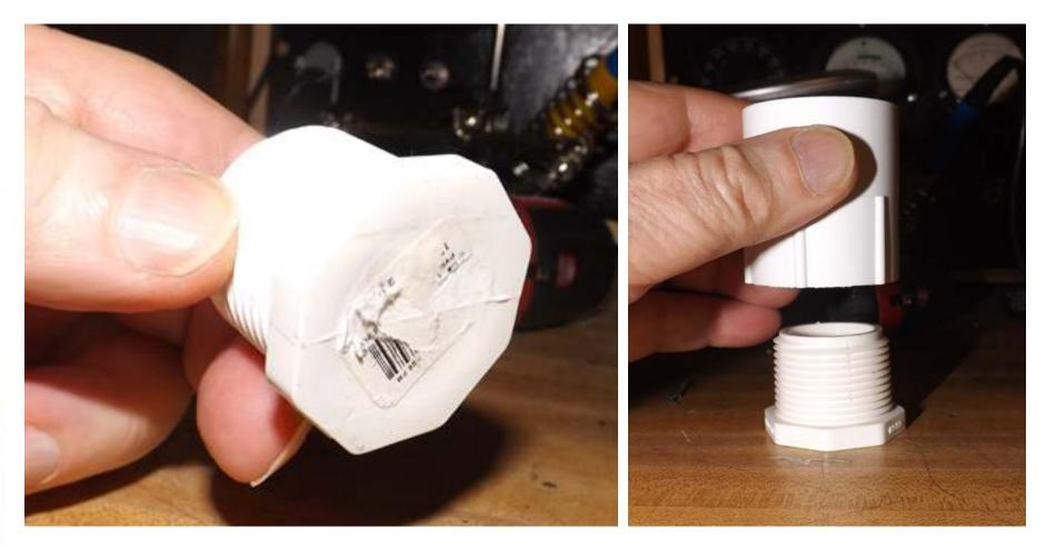
The problem here is that the plastic at the top of the plug is not thick enough to prevent rocking.
