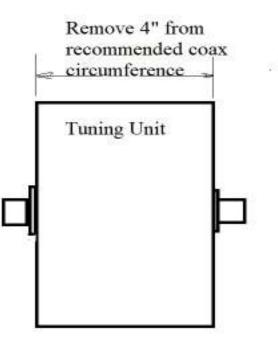
Cut coax to 96.79" before connector installation.
