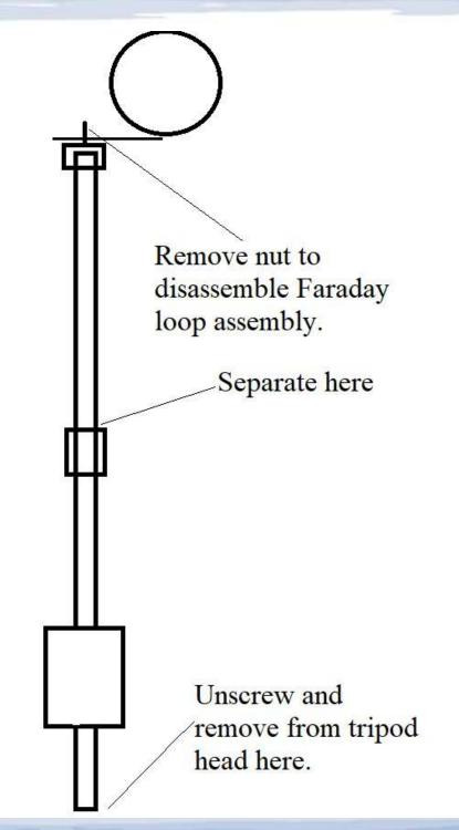
The antenna breaks down into 6 sections for storage or transporting:
