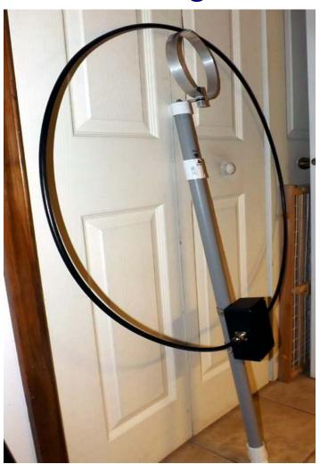
Now cut the top section of the mast to the proper height and install the Faraday loop assembly so that the top of the Faraday loop is even with the top of the main loop. Wrap the velcro to hold the tops of the two loops together.
