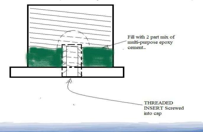
Before applying the epoxy mixture, insure that the insert is vertical in respect to the base of the cap, otherwise the antenna mast could lean off of 90 deg. vertical when mounted on the tripod.
