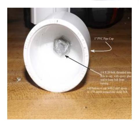
When the unit is completed and assembled, the mounting tab of the Faraday Loop will screw onto the stud protruding from the cap, and then a stainless nut and washer can be placed on the screw to secure it.
