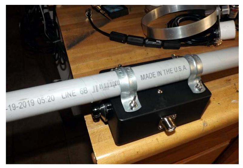
After measuring and cutting the LMR-400, and installing the connectors, the cable can be attached to the tuner in preparation for measuring the remaining section of the mast.
