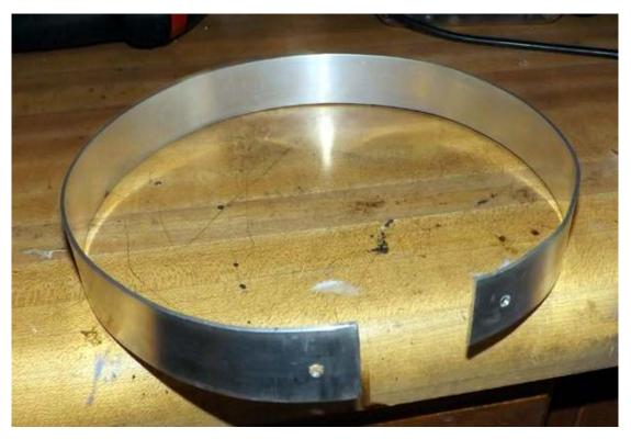
We started by cutting a piece of the 1" aluminum flat bar to a length of 23".
