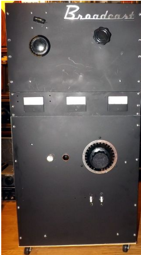
The face of the dual 813, 1 KW Grounded Grid Linear amplifier. The plate transformer is fed through a 2.5KVA Variac, which enables limiting of the output level. The red and green filament and plate indicators are from a New Orleans area power plant switchboard that my engineering company demolished back in the 1980s.
