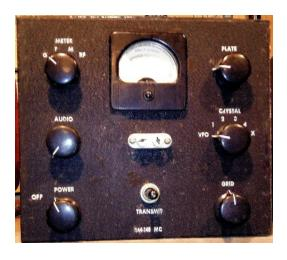
I am trying to identify this transmitter as to who made it, and any info about it. It is definitely a 2 meter AM transmitter because the front panel indicates that the frequency range is 144-148 MHz. There is no name or numbers on it, but it looks to be commercially built. The final is a 2E26
