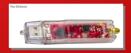
USB stick containing 70 cm data transceiver. Works with D-Star, DMR, Fusion, APCO25 and other digital modes which are based on GMSK, 2FSK or 4FSK \$150
