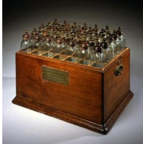
Benjamin Franklin coined the term “battery” in ca. 1749 in reference to an assembly of Leyden Jars (early dielectric capacitors)
