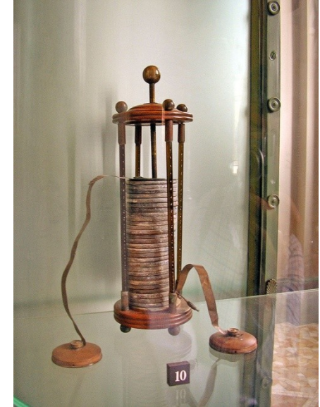
The first true primary battery was the “Voltaic Pile” developed by Alessandro Volta in 1800 containing Zn and Cu plates with a brine electrolyte.
